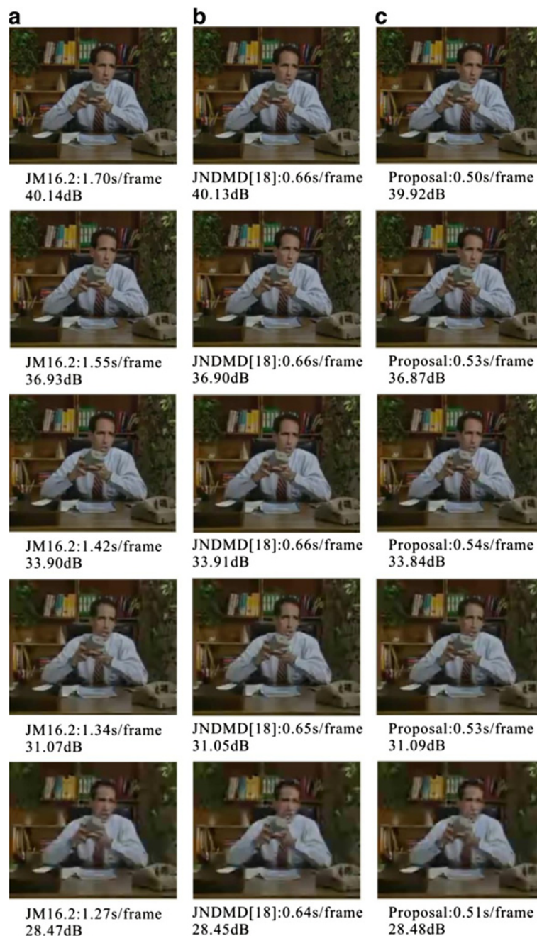
Figure 14 The subjective comparison for Salesman (QCIF) sequence (the 47th frame, IBBP): (a) JM16.2, (b) JNDMD [18], (c) proposed algorithm.
