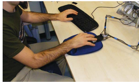
Fig. 6. Subject interacting with the mouse attached to the assistive haptic device.
