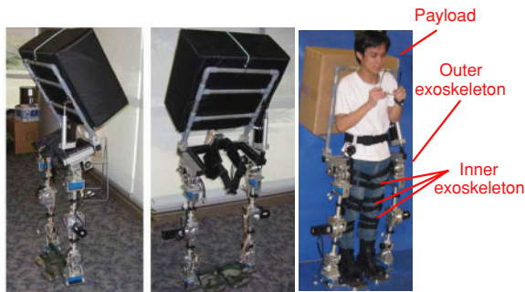
Figure 20 A user resting with the integrated exoskeleton system.
