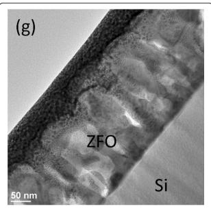
Figure 1 Low-magnification TEM image of the ZFO film on the Si.
