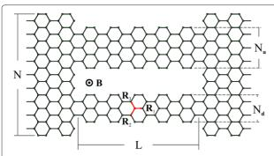
**Figure 1 Schematic view of the conductor.** Two finite armchair graphene ribbons (red lines). The length *L* of the conductor is measured in unitary cell units.
