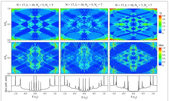
**Figure 3 Magnetic field effects on LDOS and conductance.** Contour plots of LDOS (lower panels) and conductance (upper panels) as a function of the Fermi energy and the magnetic flux crossing the hexagonal lattice for three different configurations of conductor. As a comparison, we have included the LDOS curves of the corresponding system without the magnetic field (bottom plots).
