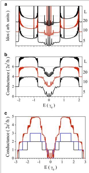
**Figure 2 LDOS and conductance for different geometries. (a)** LDOS (black line) and **(b)** conductance of two A-GRNs (red line) of widths  $N_d = N_u = 5$ , connected to two leads of widths N = 17 for different conductor lengths: L = 5, 10, 20 u.c. **(c)** Conductance of a system composed of two parallel  $N_d = 5$  and  $N_u = 7$  A-GNRs of lengths L = 15. As a comparison, we have included the pristine cases (black and blue curves, respectively).
