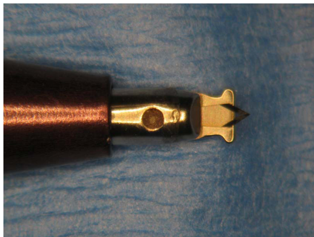
Figure 2 Accutome Rubenstein LRI knife.
