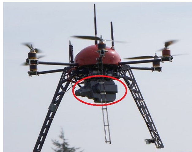
Figure 2. LOAC on board an unmanned aerial vehicle of the Fly N Sense Company; LOAC is on the black box at the bottom of the vehicle (red circle).
