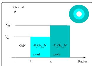
Figure 1 Structure of the spherical quantum dot and related potential distribution.
