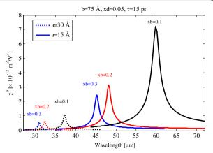
**Figure 3** Third-order susceptibility of GaN/AlGaN quantum dot versus pump photon wavelength. With different barrier potentials and defect sizes for 15-ps relaxation time.
