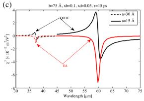
**Figure 2** Quadratic electro-optic effect and electro-absorption process susceptibilities versus pump photon wavelength. For 15-ps relaxation time,  $V_{01}=0.062$  eV. (a)  $V_{02}=0.423$  eV. (b)  $V_{02}=0.268$  eV. (c)  $V_{02}=0.127$  eV.
