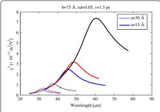
**Figure 5 Third-order susceptibility versus pump photon wavelength.** With different barrier potentials and defect sizes for 1.5-ps relaxation time (black xb = 0.1, red xb = 0.2, and blue xb = 0.3).
