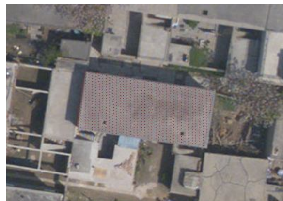
Figure 11. roof LiDAR points projected result
