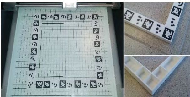
Figure 3. The standard frame called "Quadra1" during the 3D printing process.
