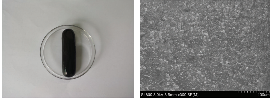
FIGURE 1: Prepared MRSP sample and SEM image of internal microstructure.
