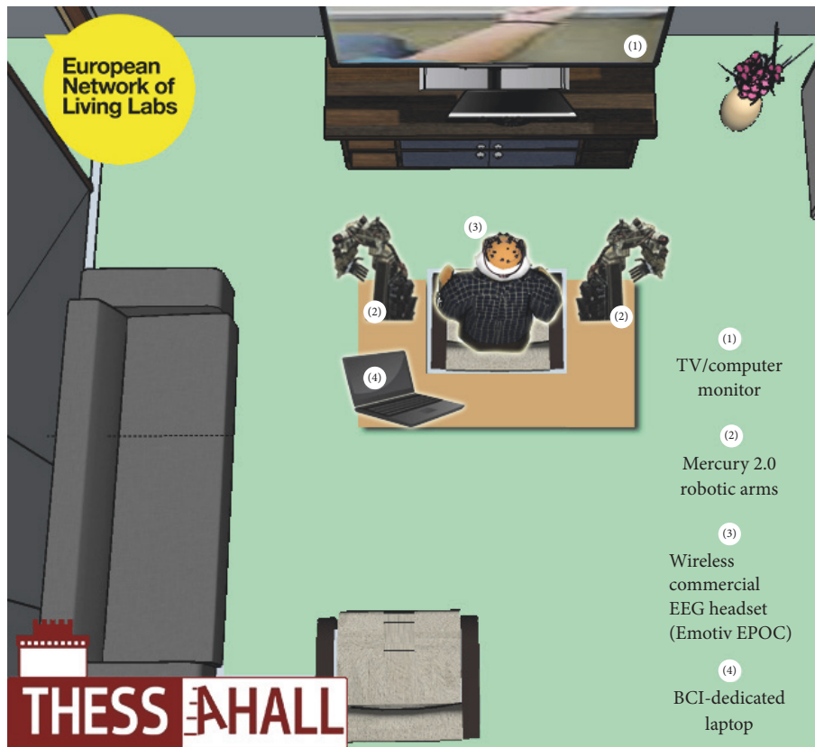
FIGURE 3: Overview of the experimental setup in the Thess-AHALL Living Lab. The figure is modified with authors' permission [46].
