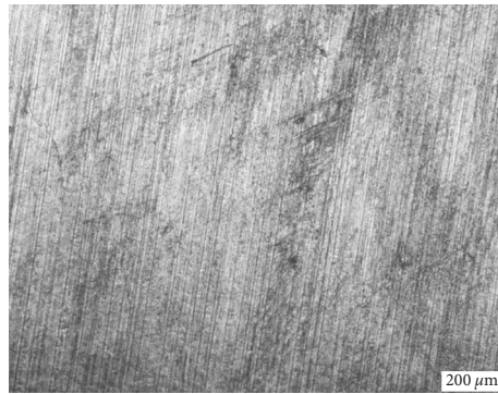
FIGURE 9: Optical microscopy for machined surface with V = 125 m/min, d = 0.30 mm, and fr = 0.05 mm/rev.
