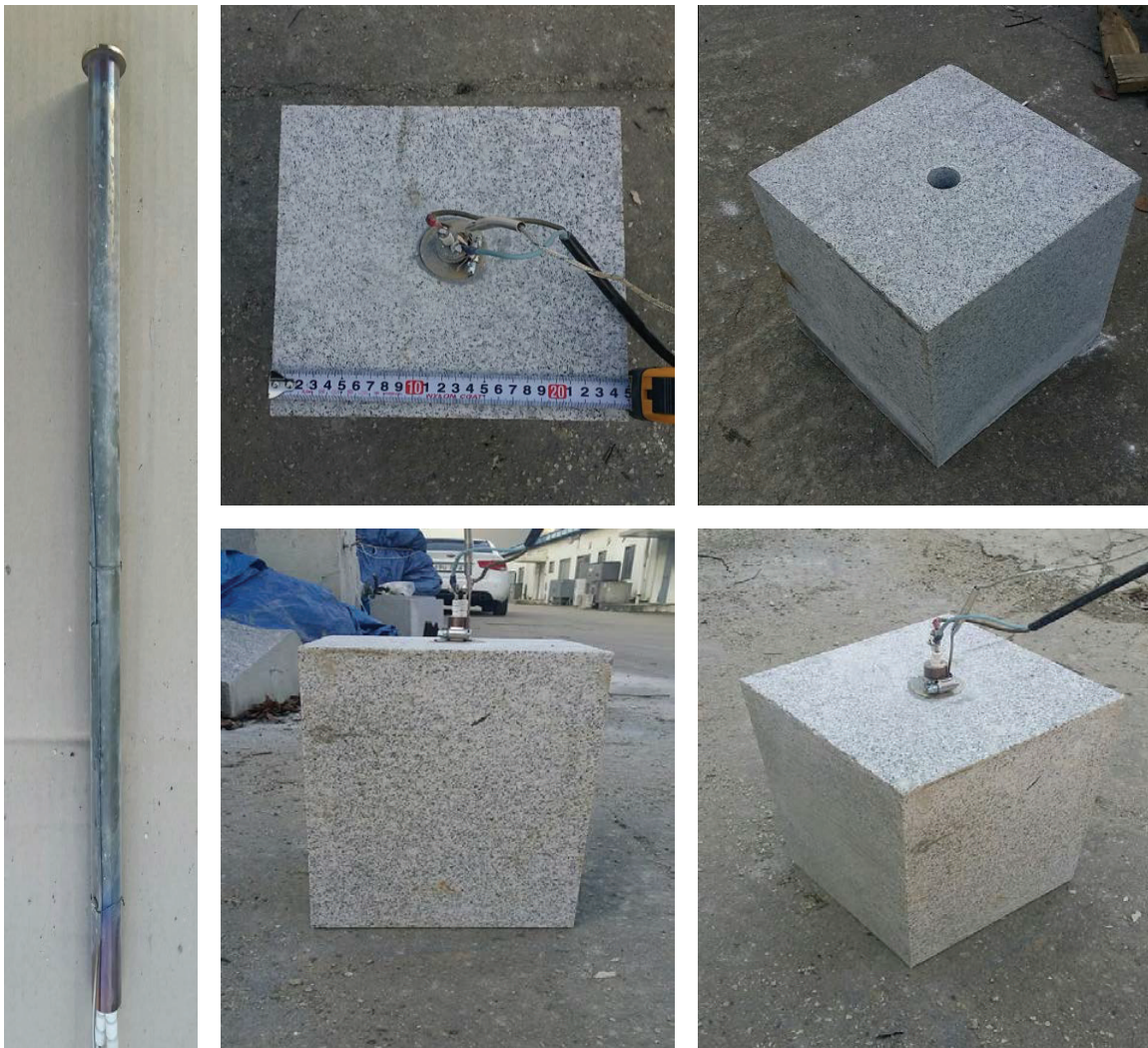
FIGURE 5: Setup for experimental field tests (heater and granite rock at the Case 1 model).
