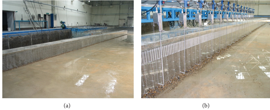
FIGURE 3: Photographs of model installation. (a) Plain wall (PW) and (b) partially perforated wall with vertical-type slits (PV_PS).
