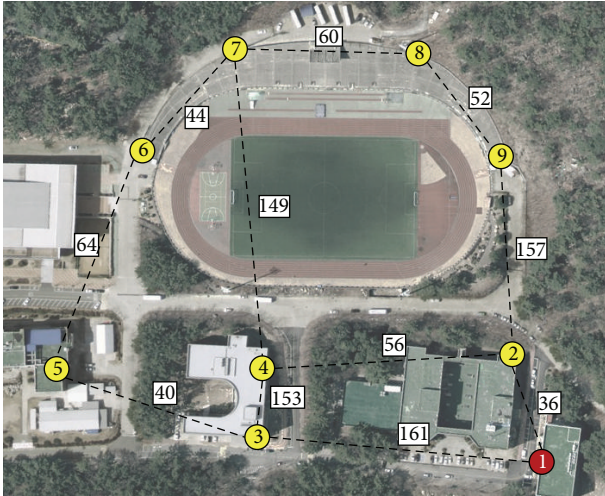
● Mesh router --- Wireless link ● Mesh portal [36] Allocated channel
