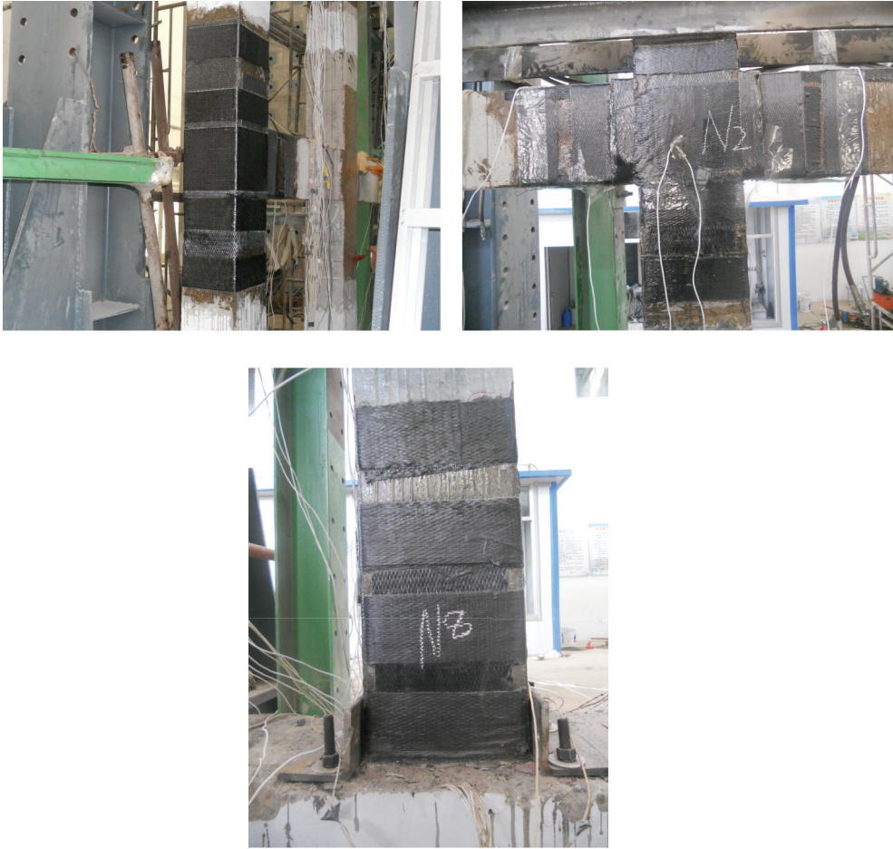
FIGURE 7: Details of CFRP sheets.
