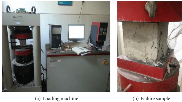
FIGURE 2: Axial compression test setup of the corroded samples.
