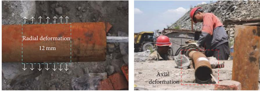
FIGURE 9: Axial and radial deformation of constant resistance casing.
