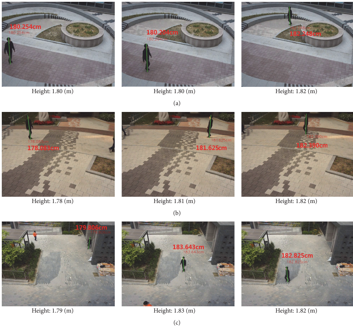
FIGURE 6: Height estimation results of the same person in three different scenes: (a) scene 1, (b) scene 2, and (c) scene 3.
