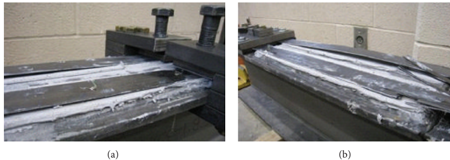
FIGURE 14: Performance of end anchorage after failure for steel beam strengthened with prestressed strips to the cover plate (a) removable end anchor and (b) fixed end anchor [68].
