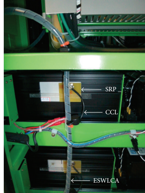
FIGURE 3: RFID sensing system with ESWLCA, CCL, and SRP for BES.
