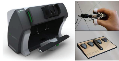
FIGURE 1: The dV-Trainer (showing console, grips, and pedals (image provided by Mimic Technologies, Inc., Seattle, WA)).
