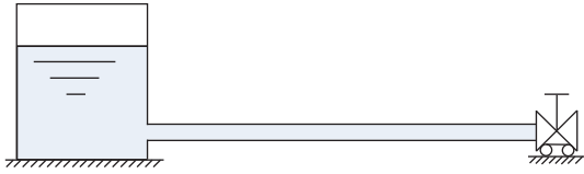
FIGURE 1: Sketch of slurry reservoir-pipeline-valve system.
