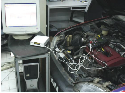
FIGURE 10: Collection of ignition patterns from a test engine using a computer-linked automotive scope meter.
