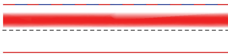
FIGURE 13: Failure modes of UHTCs which act as thermal protection materials. (Red is for tensile failure and blue is for compressive failure. Dash line indicates middle plane of the UHTC plate.)
