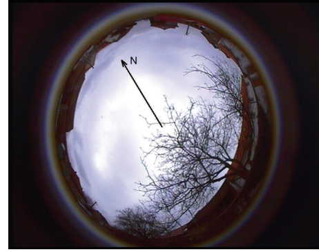
FIGURE 2: Scenario 2: the arrow indicates due north (0 deg. azimuth); the azimuth runs in a clockwise direction.
