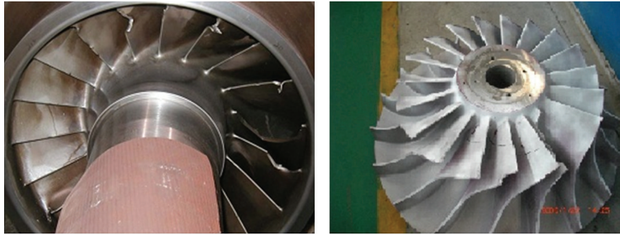
FIGURE 1: Pictures of centrifugal compressor blade cracks.
