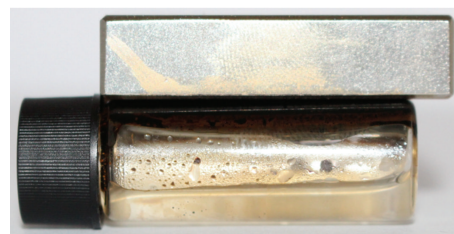
FIGURE 11: A fully phase-separated system under the influence of an external magnetic field.
