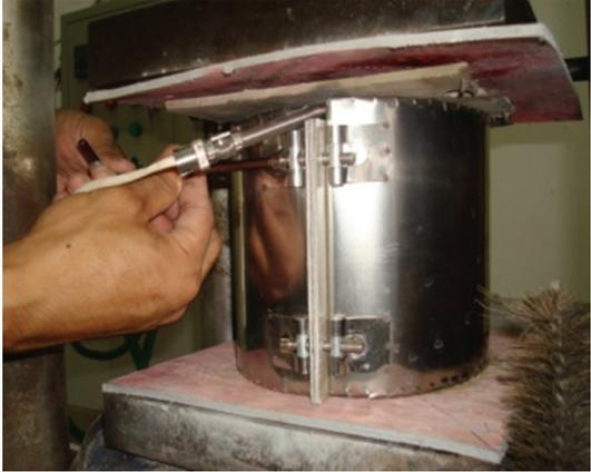
FIGURE 8: Cylindrical heating jacket.
