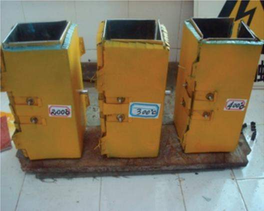
FIGURE 7: Prismatic heating jacket.
