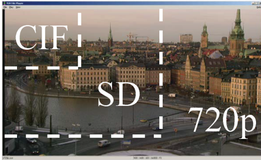
FIGURE 6: The 720 p resolution frame of the “STOCKHOLM” video sequence, which presents two ROIs having CIF and SD resolutions.
