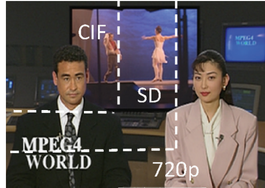
FIGURE 2: Defining ROIs with different spatial resolutions (e.g., CIF, SD/4CIF, 720 p resolutions) to be provided within a Scalable Video Coding stream.
