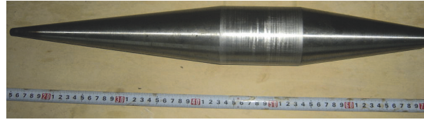
FIGURE 1: Striker of SHPB measurement equipment ( \varphi , 50 mm).
