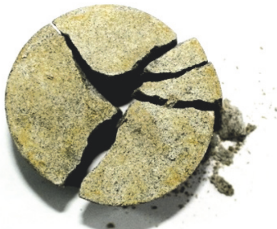
FIGURE 15: Failure modes of specimens in the SHPB test (the length-diameter ratio of specimen is 0.5, and the average strain rate is 75.3 \text{ s}^{-1} ).
