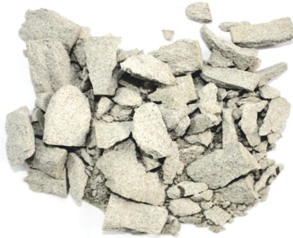
FIGURE 16: Failure modes of specimens in the SHPB test (the length-diameter ratio of specimen is 0.5, and the average strain rate is 162 \text{ s}^{-1} ).
