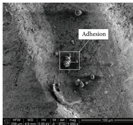
FIGURE 21: SEM micrograph of tool flank for treatment at 24 m/min and 0.15 mm/rev showing adhesion.
