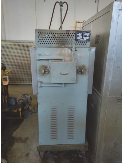
FIGURE 11: The experimental electric heating platform.
