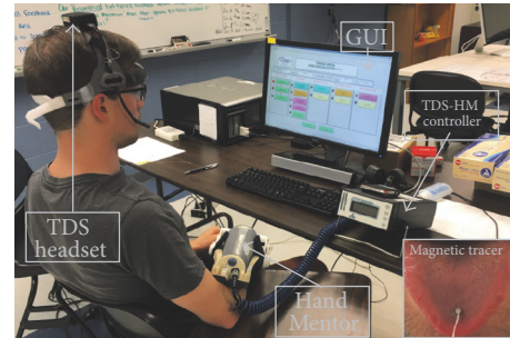
FIGURE 1: Experimental set-up. Top center, the graphical user interface (GUI) that participants view during game training. Bottom center, the Hand Mentor (HM) device worn on the right (paretic) upper extremity. Left, healthy volunteer with TDS headset affixed to the head. Magnetic sensors are positioned bilaterally to capture the maximal oral area. Bottom right, the small magnetic tracer used to control the HM device. Bottom center, the HM controller with red safety button to be used to immediately stop the training.
