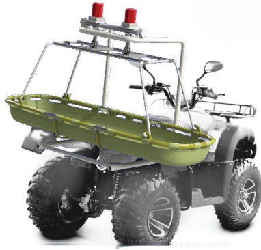
FIGURE 11: The proposal for rescuing a patient from an ATV carried on rough terrain.
