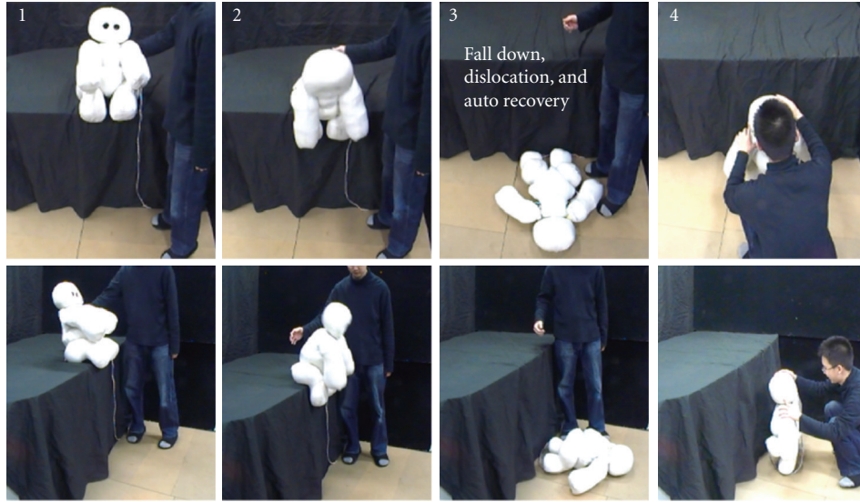
FIGURE 29: Appearance of falling down experiment by Marshmal.
