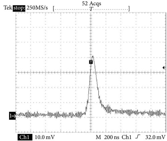
FIGURE 3: Temporal profile of the single pulse with pulse width of 108 ns.
