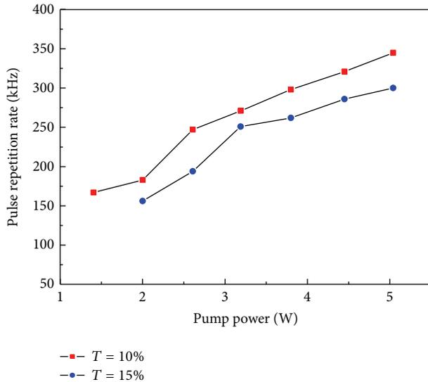
FIGURE 5: Pulse repetition rate versus pump power.
