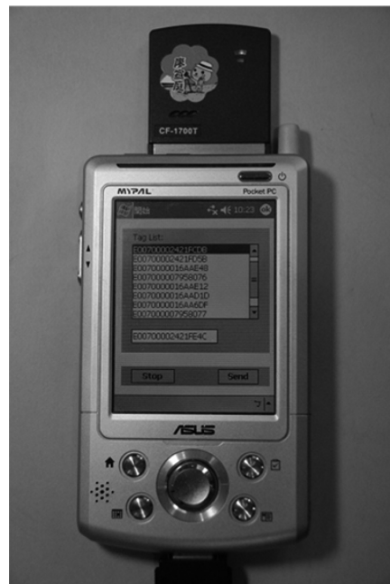
Fig. 4. The CF-card RFID reader mounted on the reader PDA.
