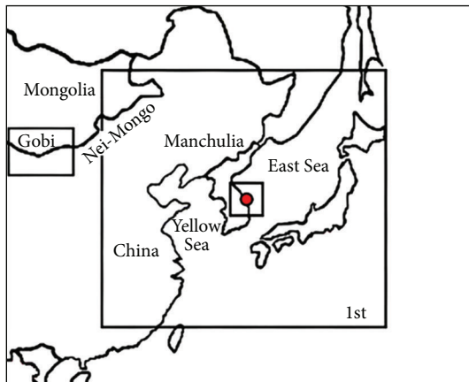
FIGURE 1: Topography of the northeastern Asia including Gangneung city ( 37^{\circ}45'N , 128^{\circ}54'E ) with the establishment of a GRIMM aerosol sampler. Large and small squares in the center indicate the first domain with a 27 km grid interval on 91 \times 91 horizontal grids and the third domain with a 3 km by three-nesting techniques in the WRF model simulation. A square in the left and a circle in the center denote Gobi Desert and Gangneung city equipped with an aerosol sampler, respectively.
