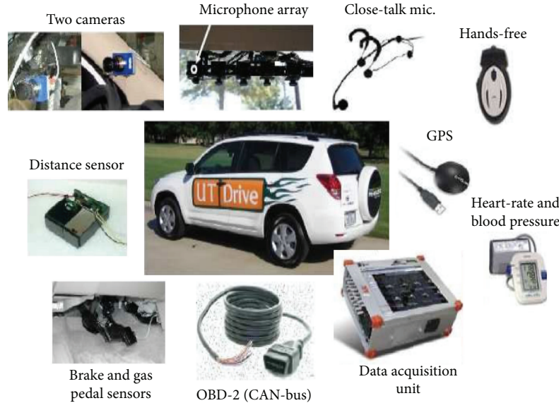
FIGURE 8: UTDrive data collection vehicle, adopted from [67].
