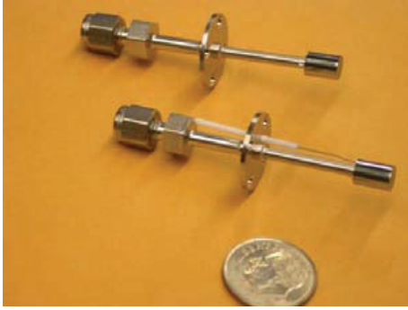
FIGURE 2: MiXI's miniature hollow cathodes.
