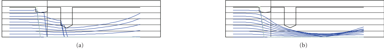
FIGURE 15: Example of beam focusing for V_B - V_A = 250 V (a) and for V_B - V_A = 550 V (b). Bottom of figures are the centerline of a axisymmetric beamlet. Results produced by CEX2D.
