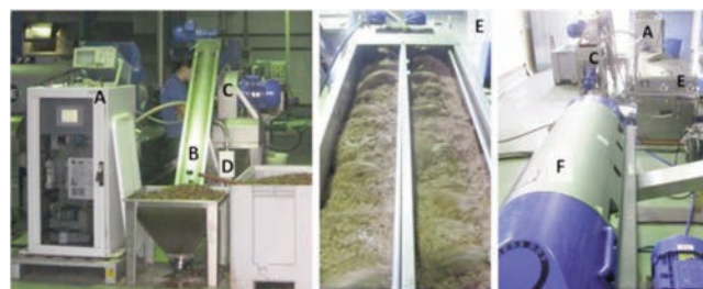
Figure 3. Setup for a pilot plant to study the PEF assisted VOO extraction process. A) pulse generator; B) Crusher feed hopper and screw; C) Crusher; D) PEF treatment chamber; E) malaxer; F) decanter.
