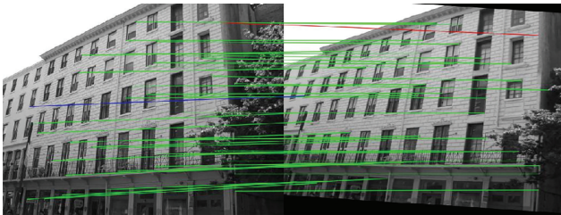
FIGURE 1: Keyframe correspondences between original and transformed images with 567 outliers. The green lines indicate correctly detected inliers, while blue means false negative and red means false positive detections. The correctly detected outliers are ignored for the sake of clearance of the figure.
