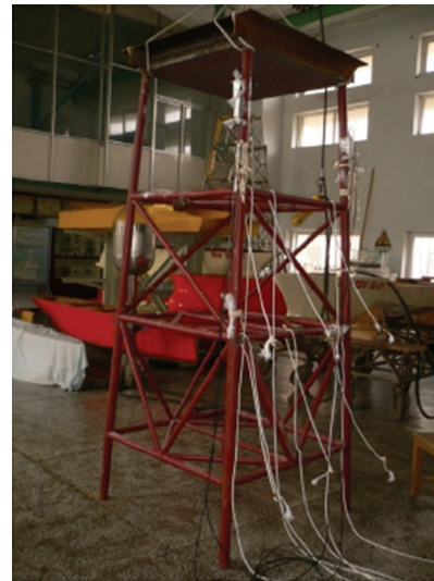
FIGURE 12: Testing model of an offshore structure.
