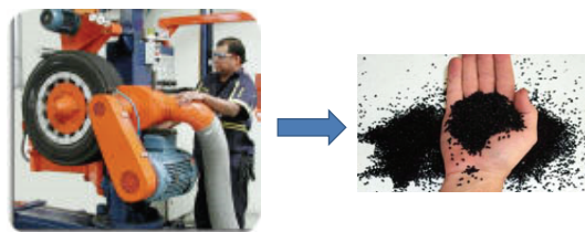
FIGURE 1: Obtaining of flake-like particles from wasted tires.
