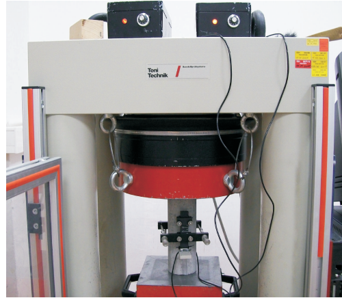
FIGURE 3: Experimental procedure for calculating secant modulus of elasticity [10] and the testing machine.
