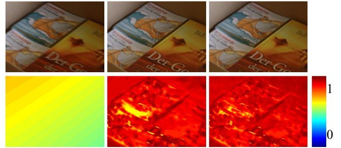
Figure 9: Visualization of pixel luckiness values at each step of our algorithm. From left to right: input blurry frame; after the 1st iteration; after the 2nd iteration.
