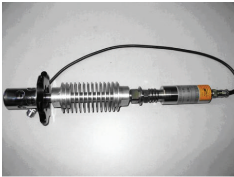
FIGURE 5: Intelligent detector of internal-combustion engine cylinder pressure with sensitivity temperature coefficient compensation-based integrated constant current.
