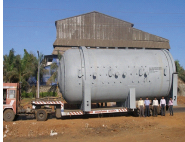
FIGURE 10: Transportation of the autoclave shell.
