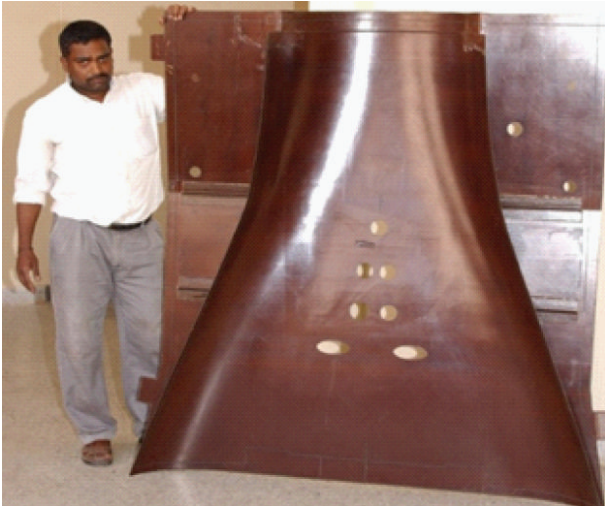
FIGURE 13: Trousers duct of LCA Aircraft cured in an autoclave at CSIR-NAL.
