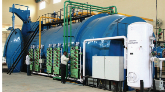
FIGURE 3: India's largest aerospace autoclave with working space of 4.4 m dia × 9 m length at CSIR-NAL, Bangalore.
