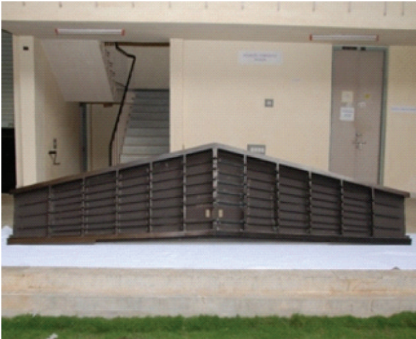
FIGURE 14: HT of SARAS aircraft, which was cured in an autoclave at CSIR-NAL.
